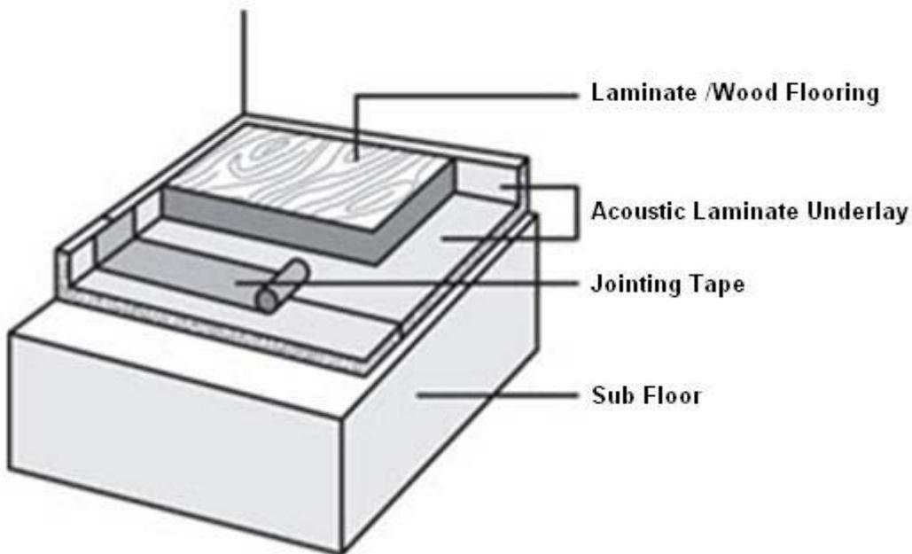
The Acoustic Laminate Underlay should be laid foil side down (essential to ensure maximum resistance to moisture from the subfloor) with each roll of underlay closely butted-up. The underlay should be trimmed-in flush to the walls. Do not use nails for this layer!
