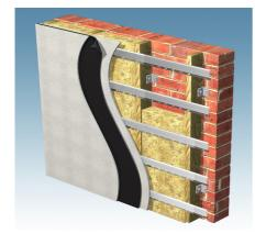
If you are experiencing loud noise such as music, we recommend using the soundproofing mats with our resilient bars. The soundproofing mat is sandwiched between two layers of plasterboard which in turn are screwed into the bars.
