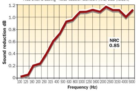
The special construction of Echosorption panels give a very high sound absorption rating 0.85 (i.e. 85%) with minimum headroom height loss of only 30mm.
