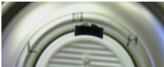
The adhesive is a contact adhesive in an aerosol can with an adjustable nozzle. You may prefer to adjust the nozzle to the widest spray pattern by pointing it to the last clockwise marking in the row of three. Then apply the adhesive to both the enclosure and the foam by holding the can about 8 inches (20cm) away and spray coat the products.
