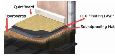
Your final hardwood floor covering should be spot bonded and secret nailed to the QuietBoard. Failure to use the QuietBoard could result in your floorboards possibly being too flexible and the floor being too soft under foot.
