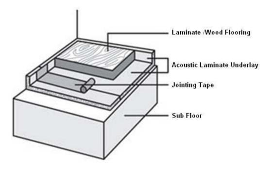
The Acoustic Laminate Underlay should be laid foil side down (essential to ensure maximum resistance to moisture from the subfloor) with each roll of underlay closely butted-up. The underlay should be trimmed-in flush to the walls. Do not use nails for this layer!
