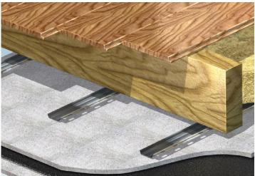
we supply, the bars will create an effective acoustic break between the bottom of the existing joists and the ceiling. If not fitted directly beneath the floor joists, Sound Reducing Resilient Bars can be supported by 50mm square battens screwed to the underside of any existing ceiling.
