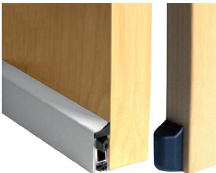
One end of the seal has a protruding plunger as shown in the picture alongside and depresses when the door is closed which activates the drop down seal that then conforms to the level of the floor and is fitted as detailed below.
