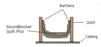
The only trimming required is to reduce the length of the product so that it sits between the joists wall to wall.
