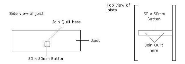
If installing within the stud frame of a wall, either the 600mm wide or 1200mm widths can be used and these are fitted in a similar way but to the sole plate, header plate and the vertical sides of the studs. In these cases, the vertical stud should be spaced at either 450mm or 1150mm depending on the width of quilt to be used.
