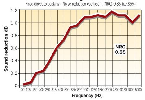
The special construction of Echosorption panels gives a very high sound absorption rating 0.85 (i.e. 85%) with minimum headroom height loss (only 30mm).
